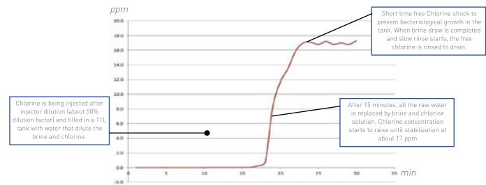
The chlorine production stabilizes after ca.22 minutes with an average value of 17ppm of free CL2.
