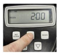
Press **NEXT.** The minutes will now flash. Use **UP** and **DOWN** to adjust if necessary
