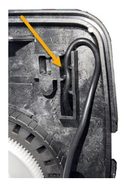
Thread the wire through the strain relief
