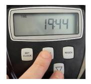
Press **NEXT** and **DOWN** simultaneously for 3 seconds
