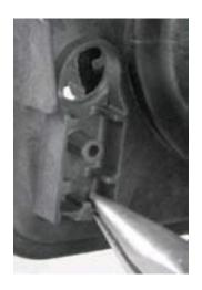
Remove the tabs at the bottom of the strain relief.
