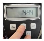
Press **NEXT** and **DOWN** simultaneously for 3 seconds
