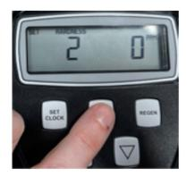
Press **NEXT** Hardness and 2 will appear. Set to "0" using **UP** and **DOWN** arrows.
