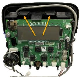
The drive bracket including PCB can now be lifted away to reveal the back plate. (Note the pictures show the meter cable which is not included with your head)
