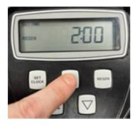
Press **NEXT.** The regen time will appear with the hours flashing. It is set to 2:00am. Use **UP** and **DOWN** arrows to adjust if necessary.
