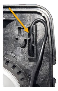
Thread the wire through the strain relief
