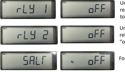
Unless you're using the relay 1 this should be set to "off"
