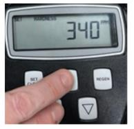
Press **NEXT** and **UP** for 3 seconds until "HARDNESS" and 340 appear. Use the **UP** and **DOWN** arrows to adjust to your hardness level\* (see notes below)
