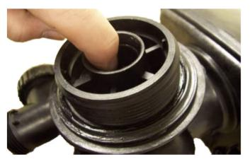
Fit the lower screen to the bottom of the valve. This is a bayonet fitting (twist to lock into place).
