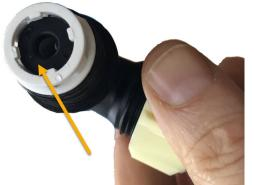
On most of the valves the DLFC is internal but easy to check. Simply pull the red tag on the drain fitting and remove the complete fitting. The DLFC is a small rubber disk with a hole in the centre located on the bottom of the fitting.
