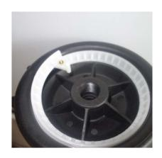
Once the end cap is in position replace the white snap ring in the groove - it snakes into position with the tab going in last.
