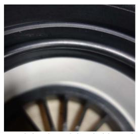
As with the other end place the lubricated o-ring on the ridge...
