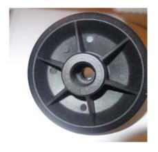
Remove the end cap from the waste/product end - this is achieved by pulling the white tab on the white snap ring. the ring will snake out of its groove and the end cap will easily pull out.
