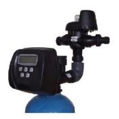
In this picture you can see a 1" / 1.25" valve with the separate source valve connected with the elbow assembly supplied, a 1.5" or 2" would have female BSP threads and would need additional pipe work to attach. The port connecting to the valve inlet would be the "C" port while port "B" connects to the untreated water and port "A" connects to the separate source supply.
